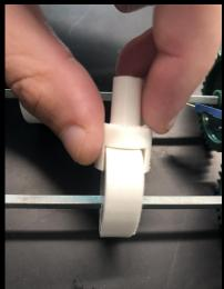
Axle holes on cam are too small - Our axle holes for our cams and pulley systems end up either too big or, more often, too small. We want our cams to be placed onto the axles but not slide once there.
